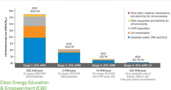
The Roadmap to Low-Cost, High-Output III-V Solar Cells
