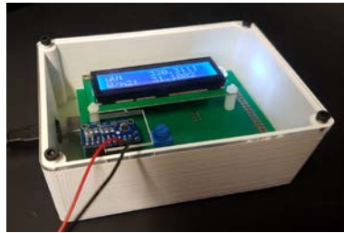
Figure 5: Arduino setup to take pyranometer readings
